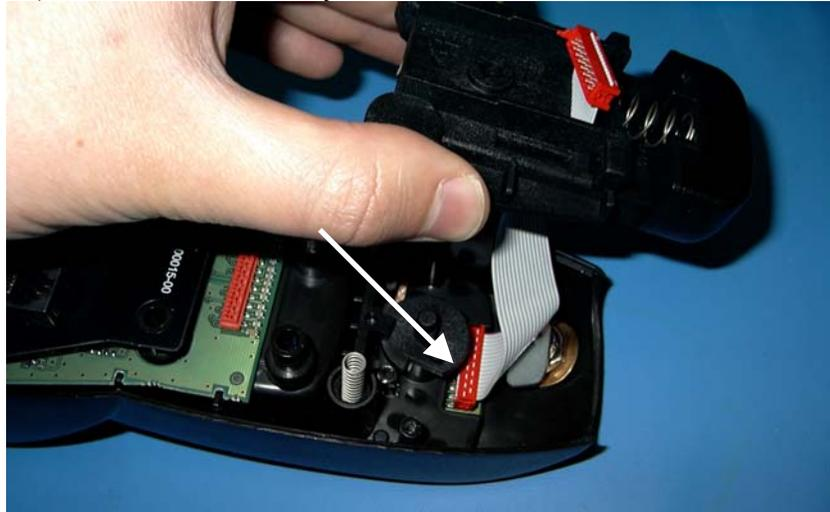
11) Hold down on the top housing and spring whilst refitting the trigger assembly cover.
